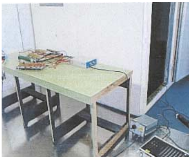
Figure A1. Conducted emissions test set-up
