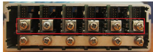
Figure 8 Minimise dV for powerMods
