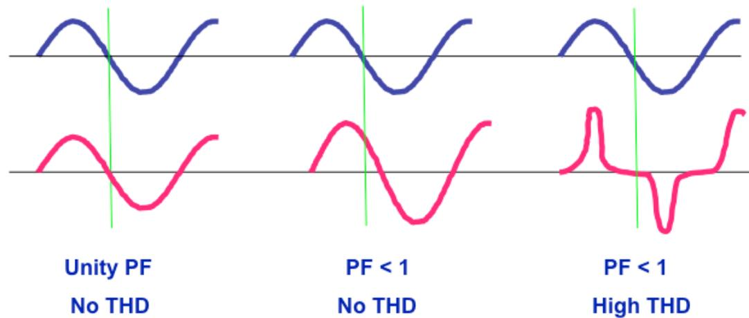
**Fig 1: Incandescent light bulbs are purely resistive load, LEDs are not.**
