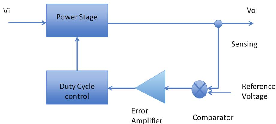
***Fig 4 : Closing the loop with a digital controller***
