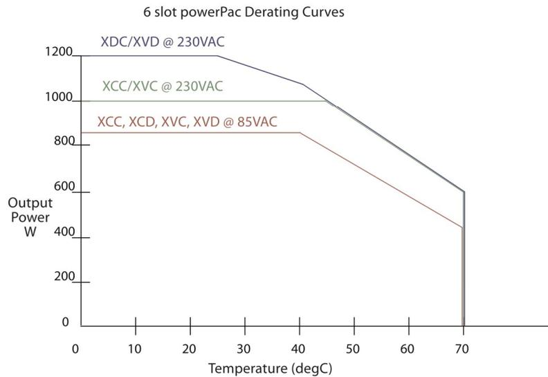
*Fig 3: Thermal derating of the Xgen series.*
