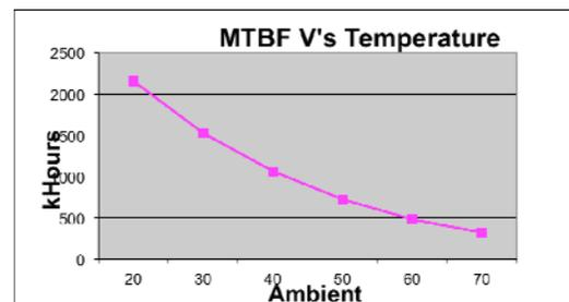
As you can see from Fig 1 above for every 10 degree rise in ambient temperature we see a 50% reduction in the calculated MTBF. This is clear if we work our way through the maths behind this.
