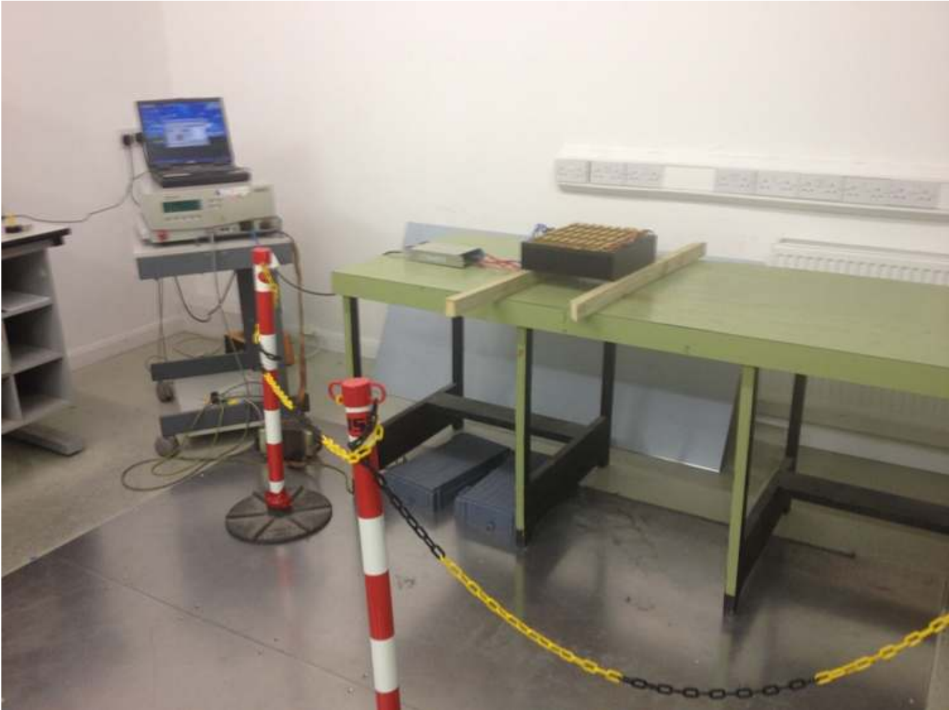
Figure 7: Surges & Voltage Dips Test Set up
