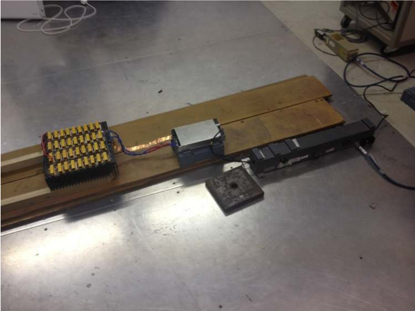
Figure 1: Conducted Immunity Test Set up
