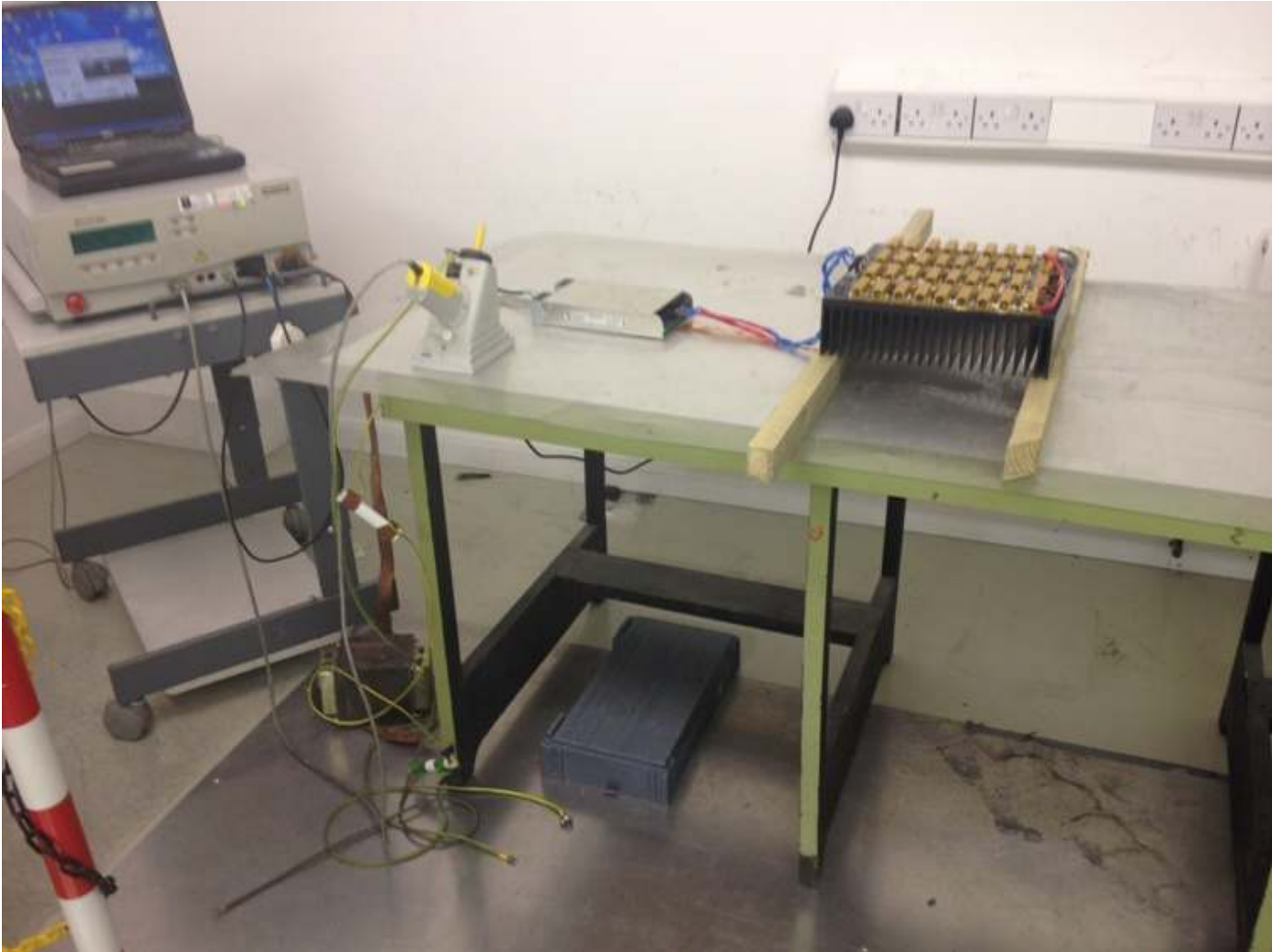
Figure 2: Fast Transients Test Set up
