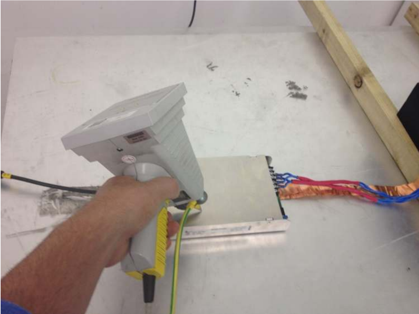
Figure 4: ESD Test set up
