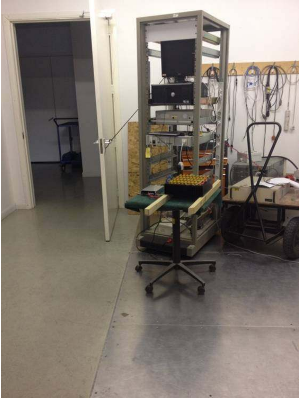
Figure 5: Harmonics and Flicker Test set up
