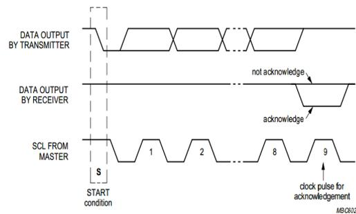
Fig.6 Acknowledge on the I<sup>2</sup>C Bus
