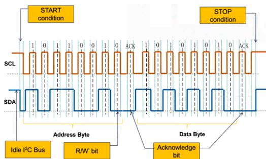
Fig.5 Transaction on the I<sup>2</sup>C Bus
