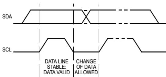
Fig.2 Bit transfer on the I<sup>2</sup>C Bus
