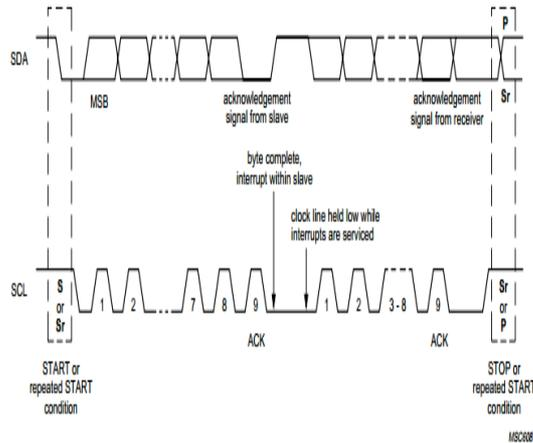
Fig.4 Data transfer on the I<sup>2</sup>C Bus
