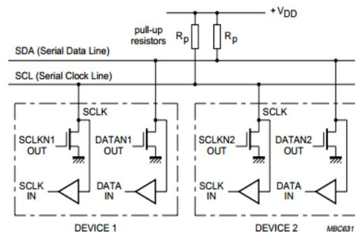
Fig.1 Connection of Standard-mode and Fast-mode devices to the I<sup>2</sup>C Bus
