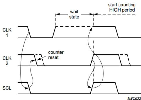
Fig.7 Clock synchronization during the arbitration procedure
