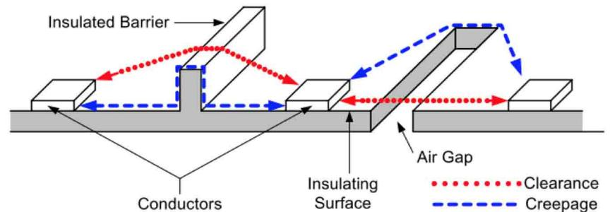
**Figure 3.** Creepage and clearance defined.
